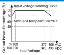
Note: ① With an AC input between 85-100V/277-305VAC and a DC input between 100-120VDC/390-430VDC, the output power must be derated as per temperature derating curves;
